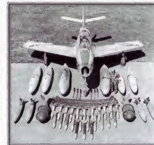
▲ Deadly arsenal The Thunderstreak could deliver a shattering array of weaponry, including rockets, 20-mm cannon fire, napalm and nuclear bombs.
